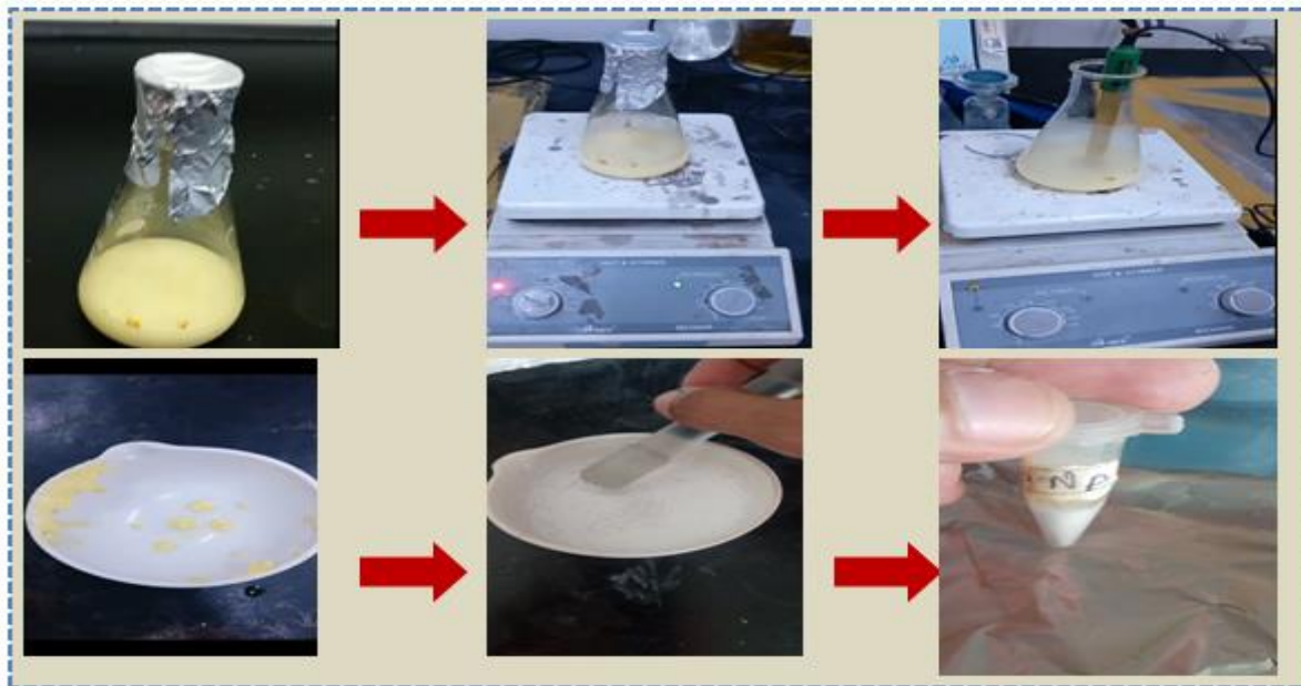
Figure 1. Shows the Titanium dioxide Nano particles Fabrication by (Top-down approach) experiment in Lab
